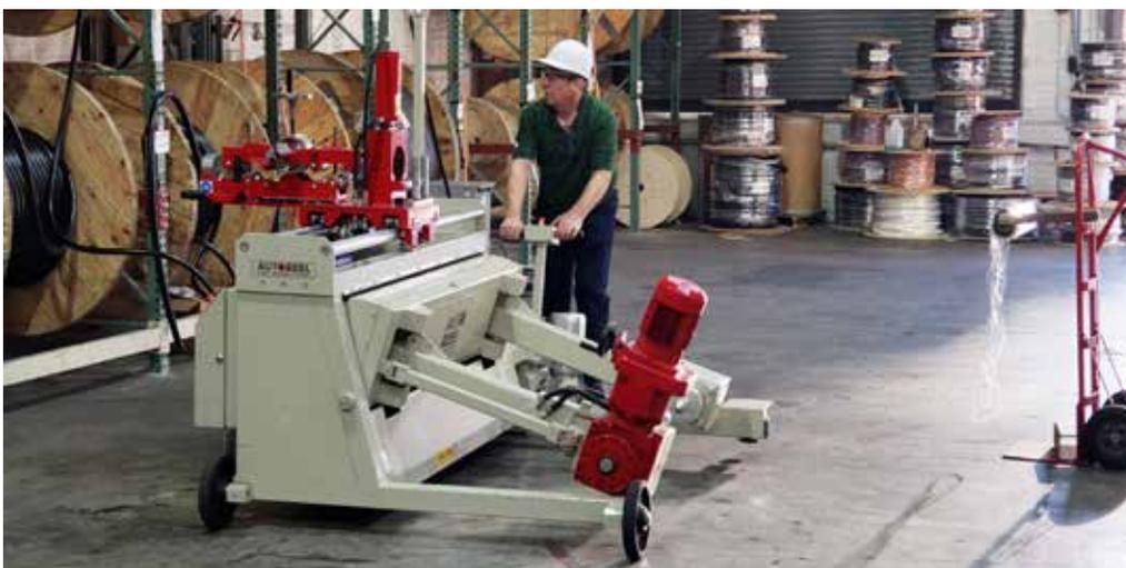
Sickler operates the wire-cutting machine.
